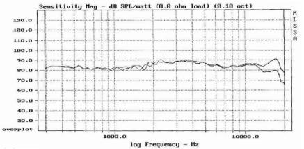
Measured on IEC baffle using Bruel & Kjaer 3144 model microp
